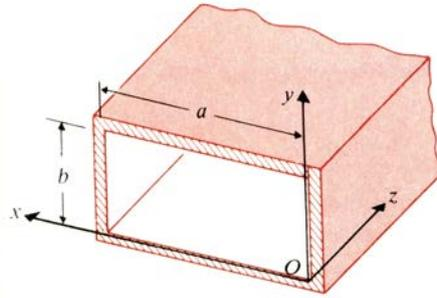
2. (10%) A metallic planar waveguide is shown as follows. What is the frequency range so that only one TE guided mode exists? Suppose the metal is a perfect conductor.
